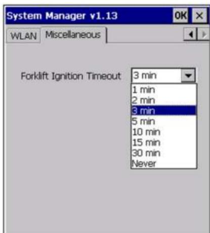
3. In the **Forklift Ignition Time-out** drop-down list, select the amount of time before the vehicle computer shuts down after the ignition switch or key switch is turned off.
